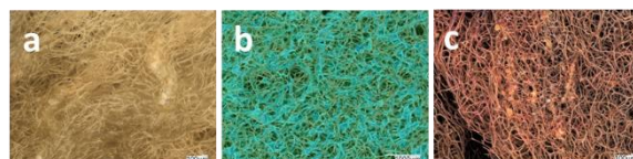
Figure 1: Optical microscope image of pure spongin (a), Sp.A (b) and Sp.Fe (c).
