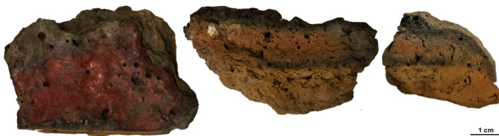
Figure 1: Cross-sections of the fragments M-F-2 (right) and M-F-19 (middle), and slagged side of M-F-19 (left).
