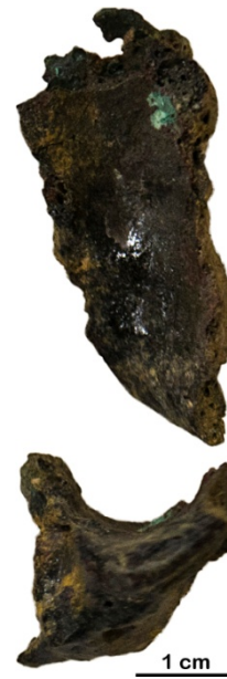
Figure 2: Entirely slagged tuyère fragment.
